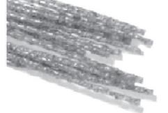
**Stripper abrasive bristle** is a 0.022” nylon filament with 120 grade grit. It is used for aggressive scrubbing and light stripping of resilient floors, terrazzo and concrete. It is as aggressive as a blue scrub pad.
